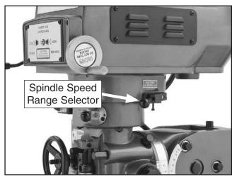
Figure 32. Model G0748 spindle speed selector.
